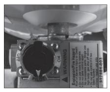
Figure 33 - Gas control/valve top view.
