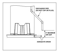
Figure 25 - Temperature and Pressure Relief Valve Pipe
