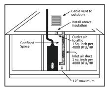
Figure 4 - Vertical duct openings
