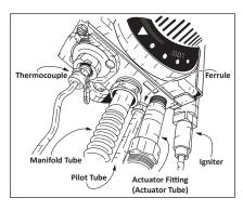
Figure 57 - Gas Valve Connections
