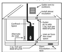
Figure 3 - Direct to outdoors openings
