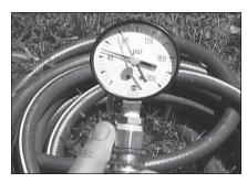
Figure 12 - Use a Water Pressure Gauge to make sure your home's water pressure is not too high.
