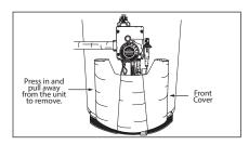
Figure 46 - Front Cover Inlet Damper.
