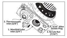
Figure 55 - New Gas Valve Ferrule Nut Removal
