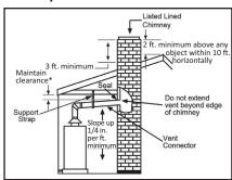
Figure 7 - Chimney termination vent system
