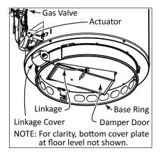
Figure 43 - Bottom view of water heater, showing actuator, linkage, and damper door.
