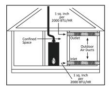
Figure 5 - Horizontal duct openings
